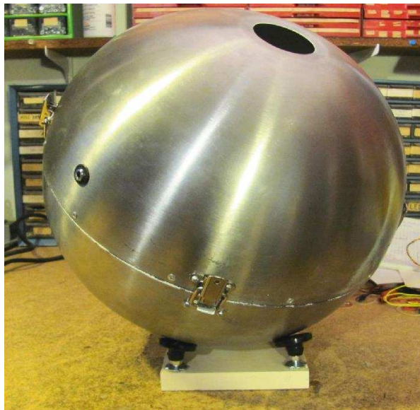
Figure 1: Integrating Sphere, showing latches, base and DC power jack for the LED light source.
