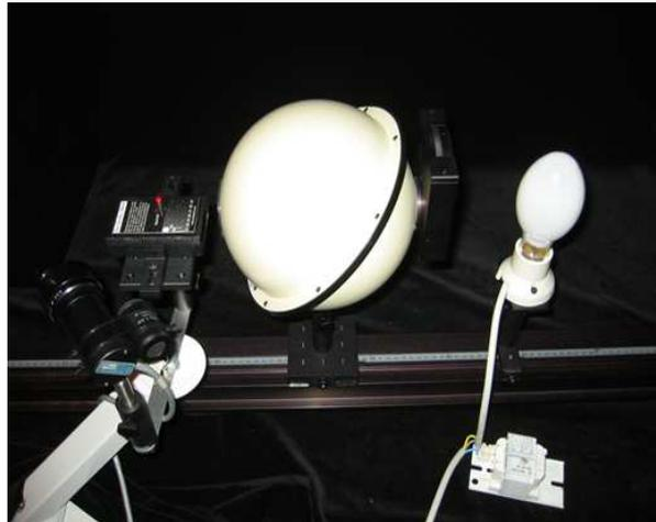
Fig. 19.— The Variable Low Light Level Calibration Standard. From left to right are visible the SQM and the reference detector, the Uniform Integrating Sphere, the aperture wheel and a test lamp for road lighting (baffles removed). Spectral irradiance/radiance standard lamps with radiometric power supplies and optical devices are used in other configurations.
